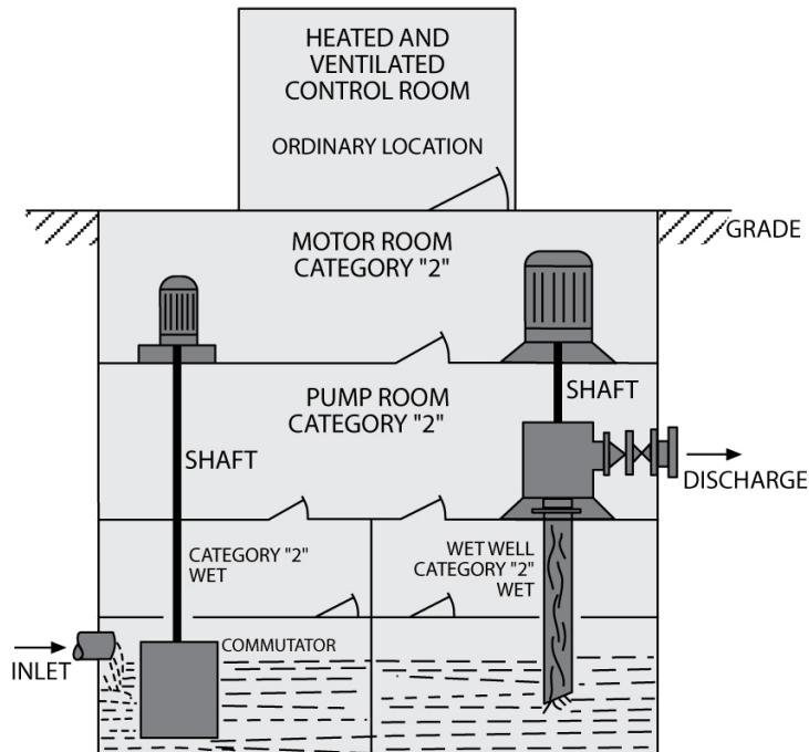
**Typical Sewage Lift Station (Side-by-Side)**
